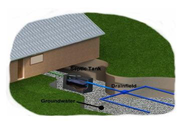
from the septic tank into a series of perforated pipes buried in a leach field, leaching chambers, or other special units designed to slowly release the effluent into the soil.
