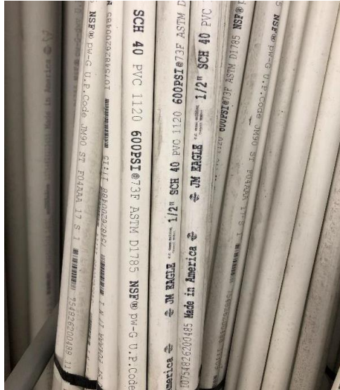
Potable white PVC line with NSF label
